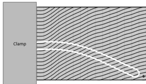
**Figure 2:** Optimal carbon fibers and SMA fibers paths. Black curve: carbon fiber path, white curve: SMA fiber path.
