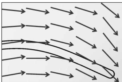
**Figure 3:** Optimal SMA fiber path and direction of the principal stress.
