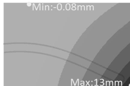
**Figure 4:** Displacement distribution when SMA fibers are activated.
